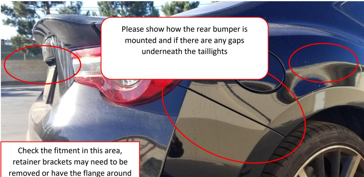
Check the fitment in this area, retainer brackets may need to be removed or have the flange around this area sanded to be inserted into the retainer brackets
